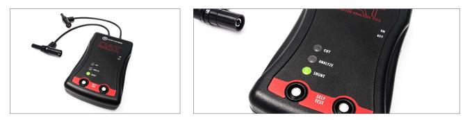
The Detonator Analysis Tool (DAT) is designed to quickly diagnose detonators in IEDs and provide the EOD operator with information that will influence the render safe procedure. It is designed for conventional EOD use on low voltage firing systems. (United States National Electrical Code rating of under 600 V) The DAT analyzes the detonator leads and provides a suggestion congruent with standard Detonator Diagnostic Truth Tables.
